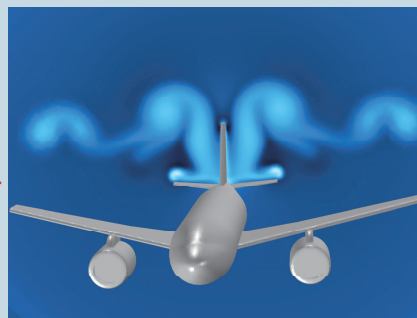
Flow around an airplane simulated with the k-ε model
