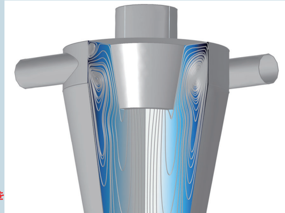
Flow in a hydrocyclone simulated with the v2-f model
